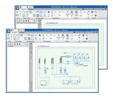
As for the refrigerant flow diagrams, **Toshiba VRF** systems can be introduced in the program, as heat pump or 3-pipe heat recovery systems. When the program performs the analysis, it checks all the maximum pipe lengths, elevation changes and working ranges, and are justified with a report.
