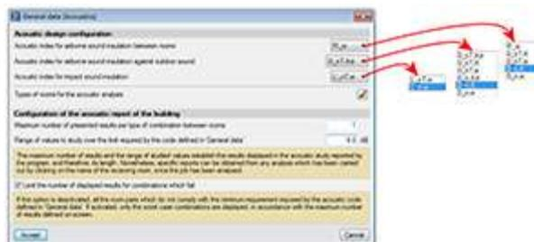
The room or precinct type definition process for the acoustic design contains a library system in the hard drive, where users can import and/or export the configuration in each job or mark a default configuration for new jobs. This way, the different acoustic standards due to different countries or project types, must only be configured once.
